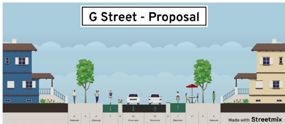
Equitable space allocation for G Street, providing people-oriented space for walking, biking, rolling and socializing while maintaining access for vehicles
