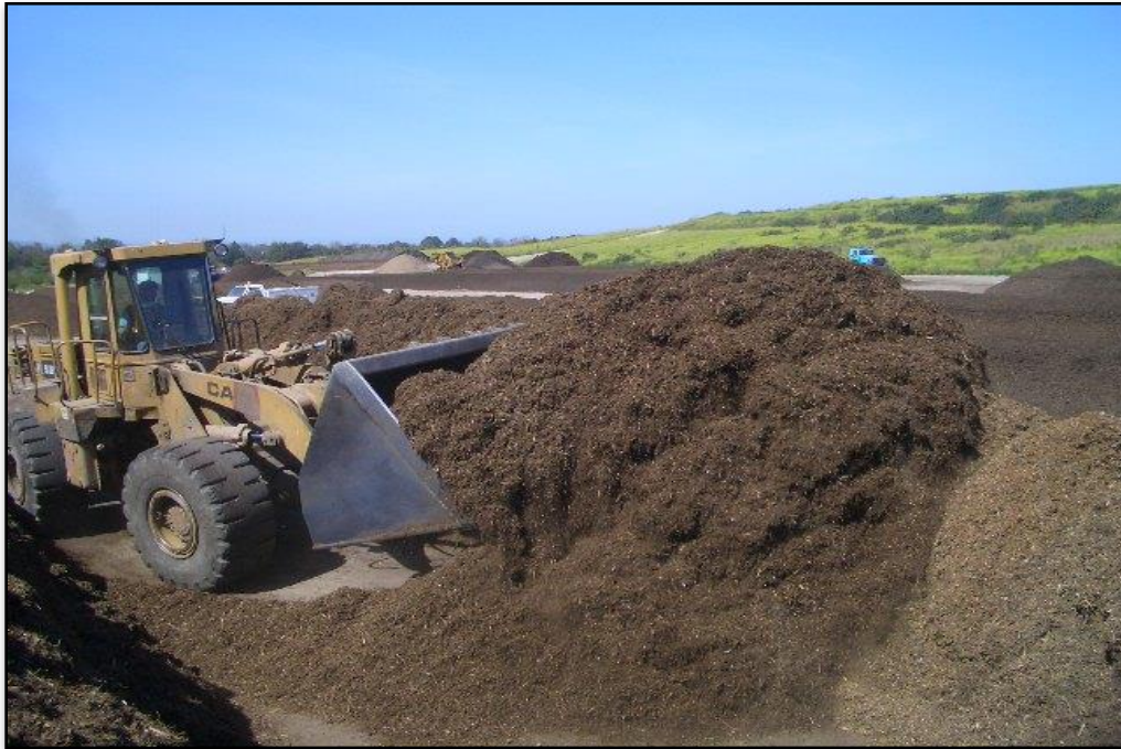
Figure 6.10 Example Static Pile Composting Pile Formation (Source: Tierra Verde Industries)
