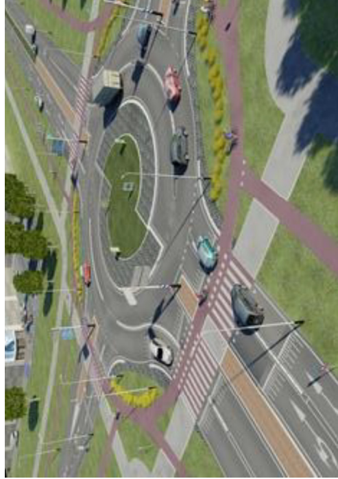
10: Turbo roundabout: Narrow, double lane but without weaving conflicts. Cyclists and pedestrians cross on a platform, with right of way.
