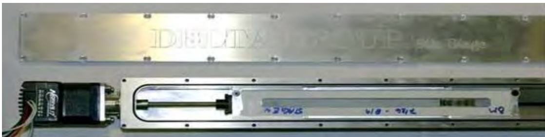
Figure 7. Continuous Ultra-fine sampling system (DRUM stage 9)
