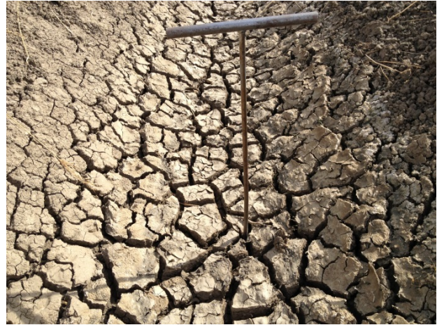
Desiccation Cracking in Irrigation Ditch
