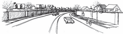
Minimal Landscaping and Inadequate Openings for Access
